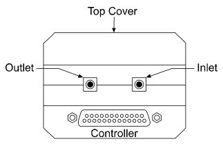
Figure 7. Coolant Ports
